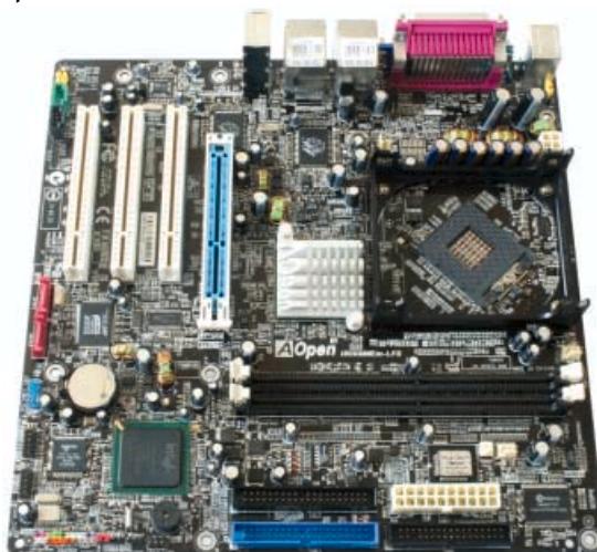
Aopen's i855GME-LFS is the first desktop motherboard designed to take the Pentium M processor
